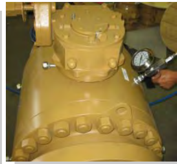
Cavity relieve pneumatic inspection at ISV
