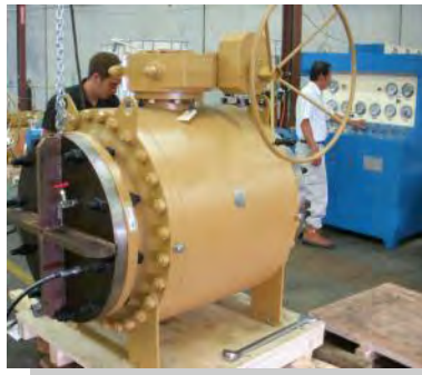
API 6D test inspection at ISV-Stafford: Hydraulic shell & seats, pneumatic seats, double block & bleed test.
